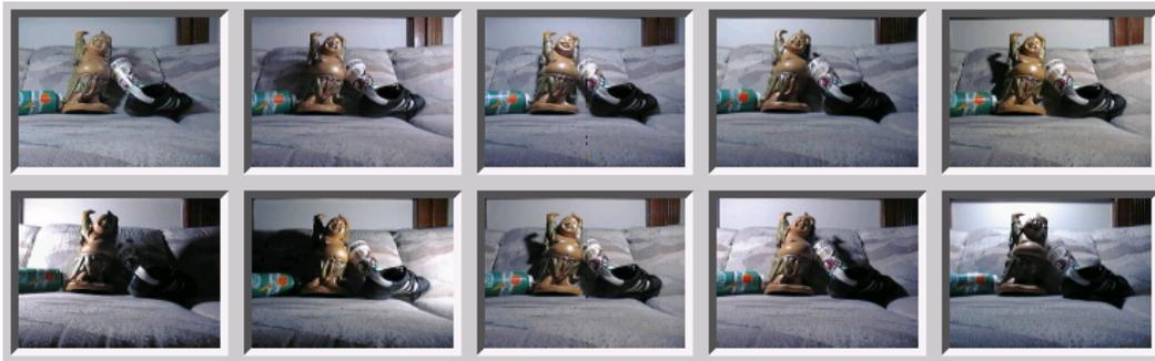
Figure 5-26: The 10 target images used to measure performance with respect to larger variations in light position, which cause hard shadows
