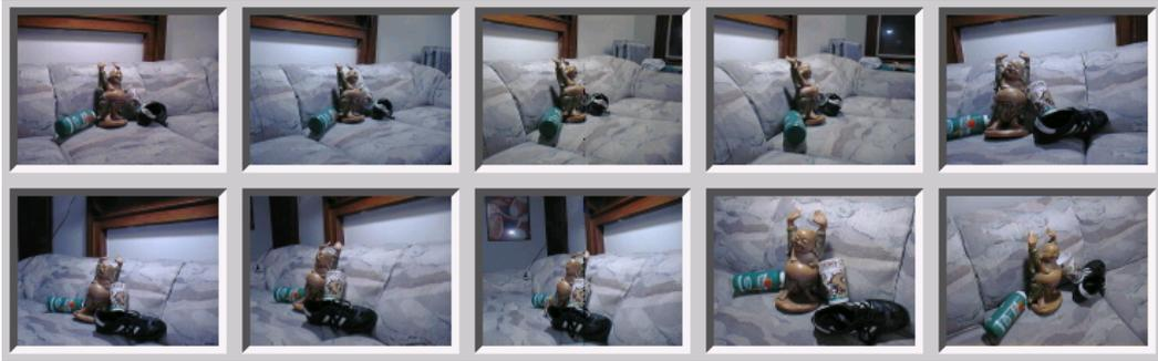
Figure 5-22: The 10 target images used to measure performance with respect to variations in camera position
