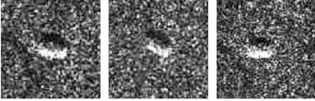
Figure 3. Target chips synthesized by sampling directly from the probabilistic distribution generated by the flexible histogram model generated from several example vehicles.
